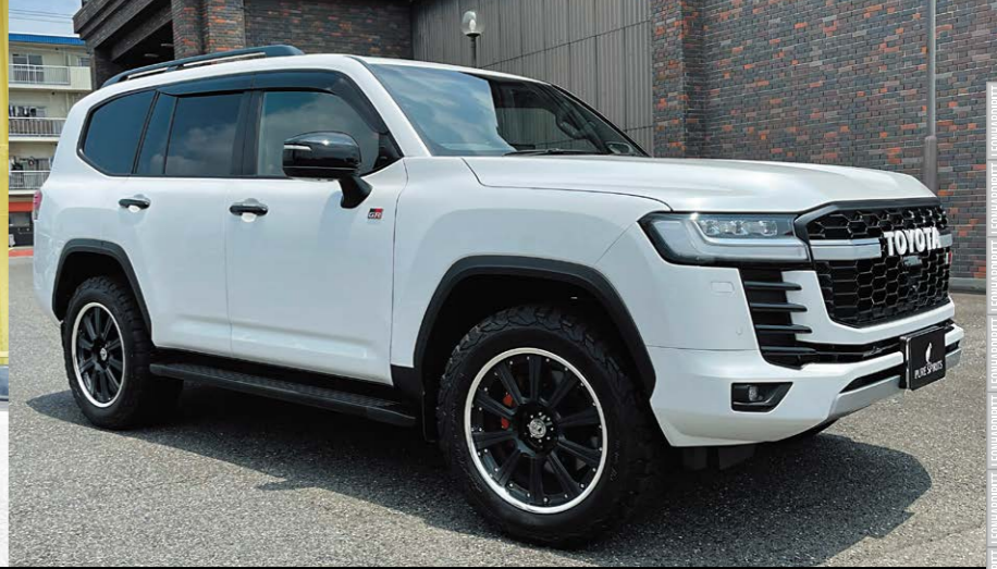
TOYOTA LAND CRUISER (300) GR SPORT COLOR: DESERT BLACK REVERSE RIM P.C.D.: 6-139.7 SIZE: F/R 2095 INSET 53 275/55-20
